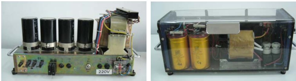
Fig. 8.13 Other DC sources achieved in the Power Electronics Laboratory with single-phase full-bridge rectifiers, capacitive filters and braking circuits.
